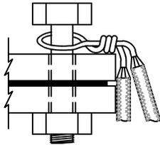
TO PUT CONTINUOUS TRACE WIRE UNDER BOLT, FIRST LOOSEN BOLT, THEN STRIP 3" MIN., WRAP ONCE AROUND BOLT, 1 TWIST, 2 WRAPS. "DO NOT CUT WIRE" TIGHTEN BOLT AFTER WRAPPING TRACE WIRE AROUND THE BOLT.
